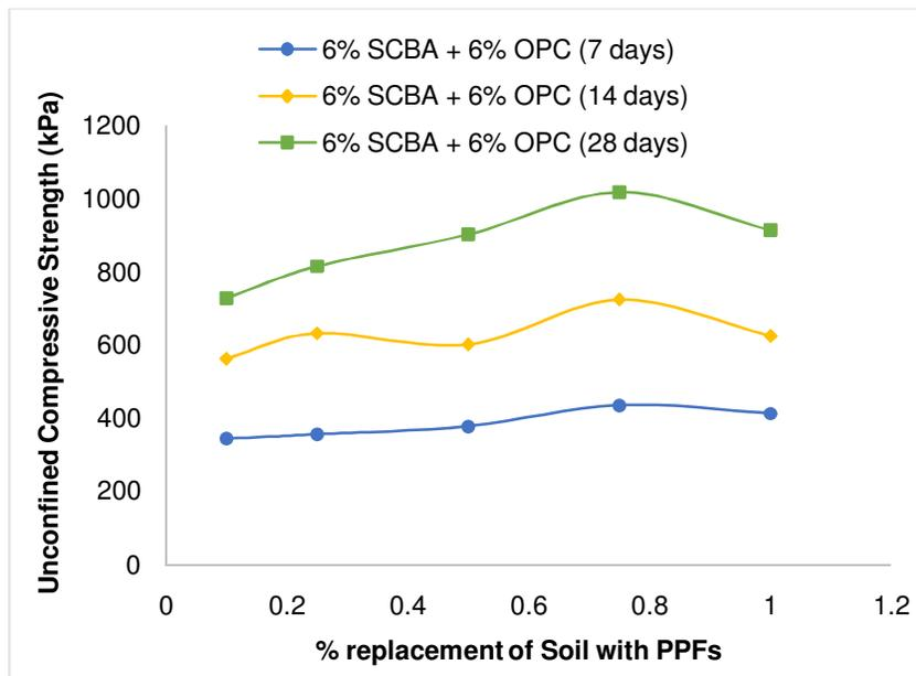
**Fig. 13.** Variation in UCS with a curing period of Soil/Cement/Bagasse ash/PPF mix.
