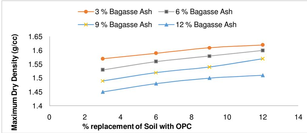
**Fig. 8.** Variation in MDD with cement content for soil-cement-bagasse ash mixtures.
