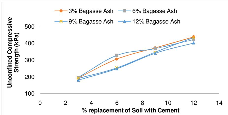
**Fig. 10.** Variation in UCS (14 days) with cement content for soil-cement-bagasse ash mixtures.
