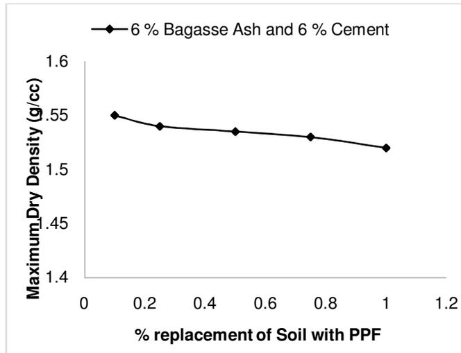
Fig. 11. Variation in MDD with PPF content in optimum soil-cement-bagasse ash mix.
