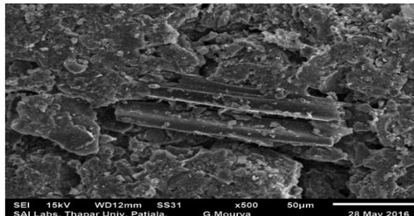
**Fig. 16.** SEM image of Soil/SCBA/OPC(88:6:6).
