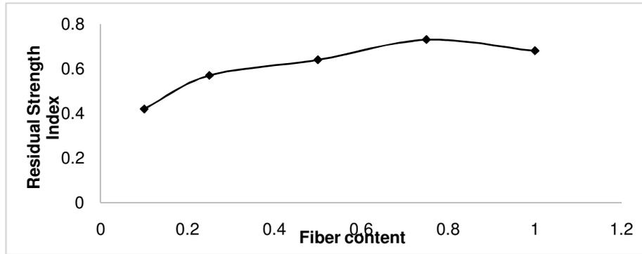
**Fig. 14.** Variation in Residual Strength Index with PPF content in Soil/SCBA/OPC mix.
