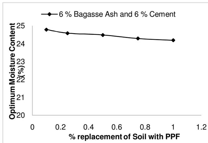
Fig. 12. Variation in OMC with PPF content in optimum soil-cement-bagasse ash mix.
