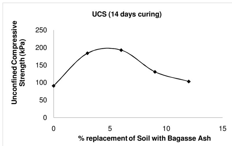
**Fig. 4.** Variation in UCS with % replacement of soil with Bagasse Ash.
