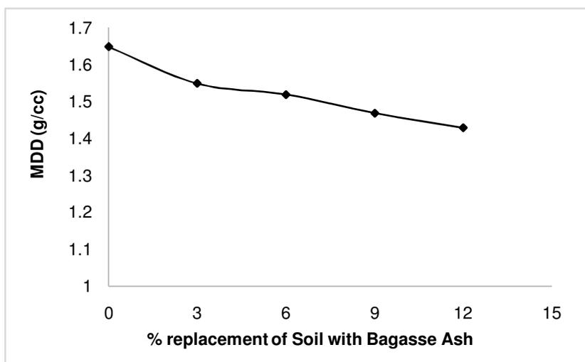
Fig. 2. Variation in MDD with % replacement of soil with Bagasse Ash.
