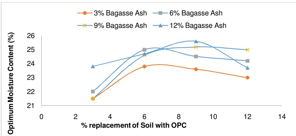
**Fig. 9.** Variation in OMC with cement content for soil-cement-bagasse ash mixtures.
