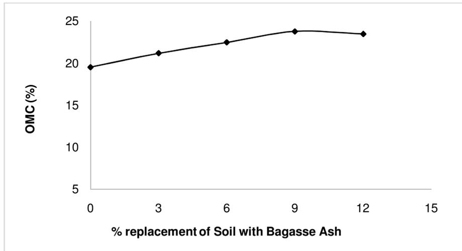
**Fig. 3.** Variation in OMC with % replacement of soil with Bagasse Ash.
