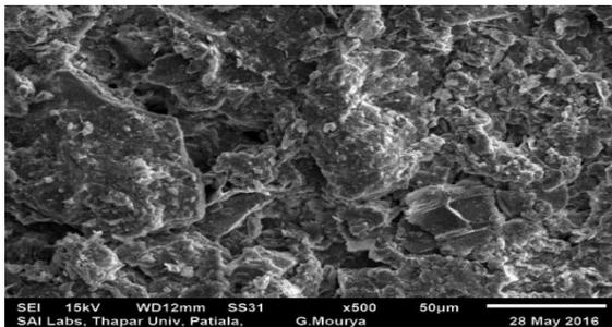
**Fig. 15.** SEM image of clayey soil.
