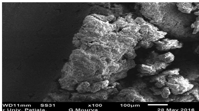
**Fig. 17.** SEM images of fiber-reinforced bagasse ash-cement mix stabilized soil (6% Bagasse ash, 6% Cement and 0.75% fibers).
